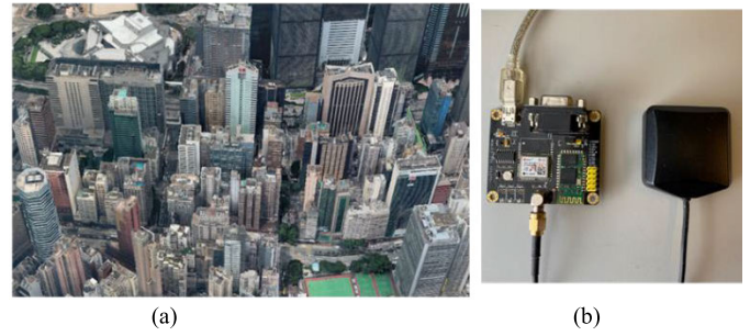
Fig. 4. (a) Experimental environments. (b) GNSS devices: U-blox M8 and antenna.
